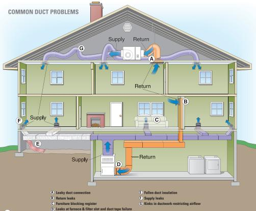
Improve your ducts by sealing leaks and insulating the ducts in attics and crawl spaces. This will improve your system's overall performance and your home's comfort and indoor air quality. You should have your duct system checked by a professional contractor to ensure it is operating efficiently to deliver the right amount of conditioned air.
